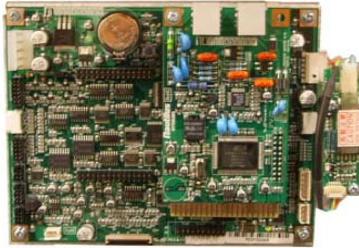
Fig. 3.7 Main Control Board
