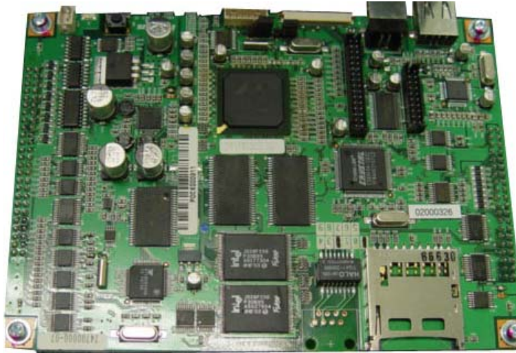
Fig. 3.8 Main Control Board
